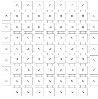
Fig. 1. FPGA architecture of matrix structure
