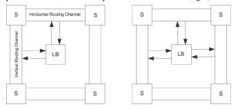
Fig. 3. Input/outputs pad of the logic group
