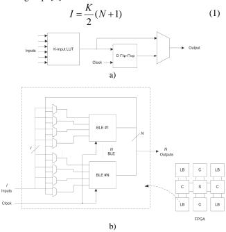
Fig. 2. BLE structure (a) and a logic group (b).
