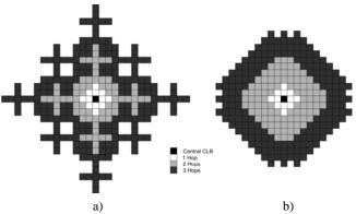
Fig. 8. Interconect Pattern for Virtex-4 (a) and Virtex-5 (b).
